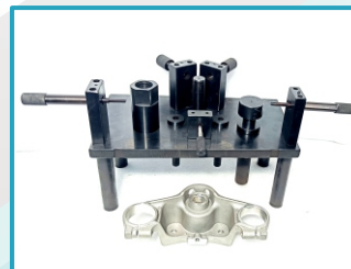
RELATION GAUGES FOR CROWN HANDLE
